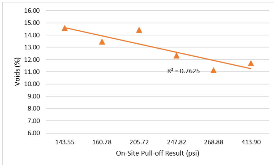
Figure 5-4. Relationship between voids and on-site pull-off result
