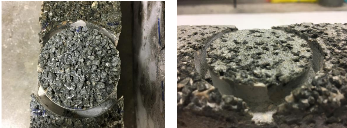
Figure 4-14. The top surface of the EO beams for pull-off test: surface before grinding (left) and surface after grinding (right)
