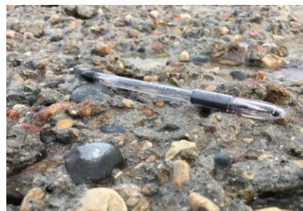
Figure 4-6. The texture of the substrate slabs: the lab substrate slab (upper), the deck substrate after milling (bottom left) and the deck substrate after hydro-demolition (bottom right)
