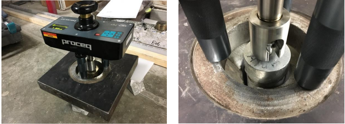
Figure 4-13. The pull-off test mounting device and the mounting detail: the mounting device (Proceq DY-216 model) (left) and the mounting detail (right)
