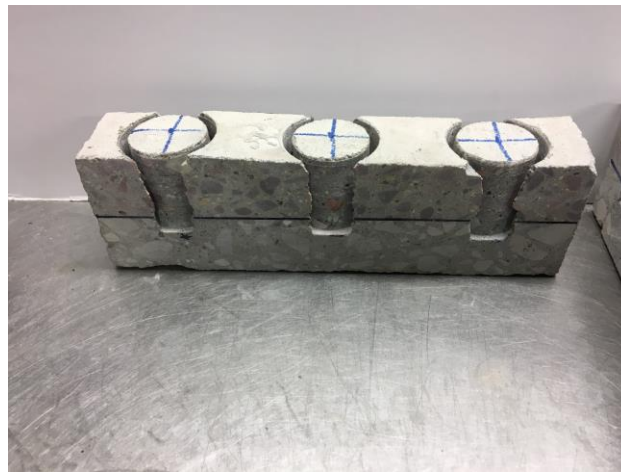
Figure 4-12. The CO beam with two-inch circular cuts
