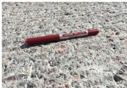
Figure 4-6. The texture of the substrate slabs: the lab substrate slab (upper), the deck substrate after milling (bottom left) and the deck substrate after hydro-demolition (bottom right)
