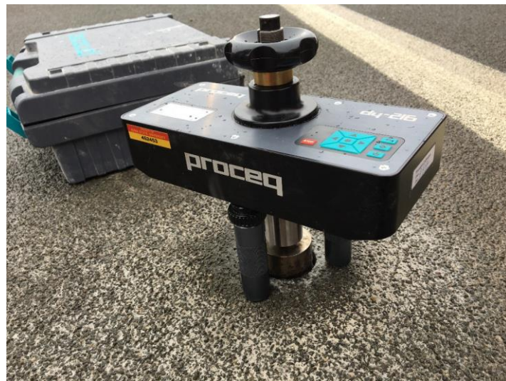
Figure 3-13. The pull-off test mounting device
