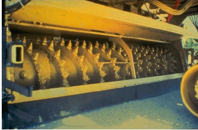
Figure 2-5. Drum of a cold-milling machine
