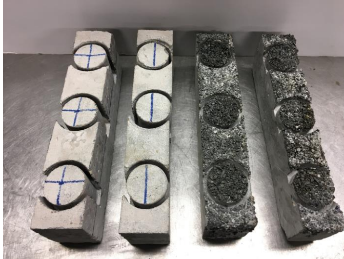
Figure 4-11. The CO and EO beams prepared for pull-off test
